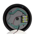
Remove the battery cover and install the batteries provided (most models have 3 batteries; some have 4 batteries). Replace the slide-on battery box cover and snap it into place. There is no screw needed. Use AA Solar Rechargeable NiCd, 1000 mA only (DO NOT use standard AA batteries.)
