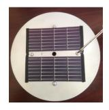
Using a Phillips screwdriver, remove the 4 Phillips screws on top of the solar light.
