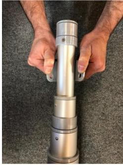
For 25' poles, remove the double harness from the top harness. Remove the spring clips. Open the double harness and attach to the top section underneath the retainer ring. This will require some force, but will not damage the double harness. Attach spring clips to double harness.
