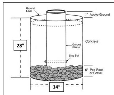
Push the sleeve into the gravel while making sure that the ground sleeve is at least 1" above ground level.
