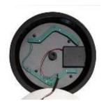
Lift off the top solar cover of the light and set down next to the bottom section, being careful not to disconnect or damage the wiring.
