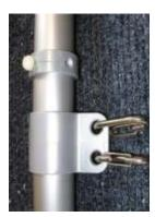
After attaching your flag, the stop ring will work best about 2" *above* the double ring. Tighten down the white thumbscrew by hand, to hold in position.
